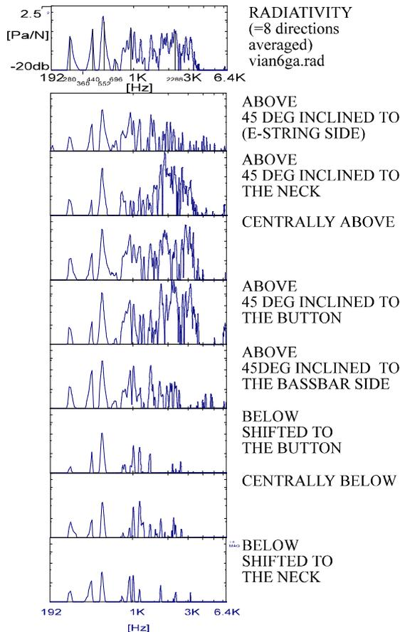
Fig. 2. The radiativity and the frequency response functions (H1,MAG) for different microphone positions.
