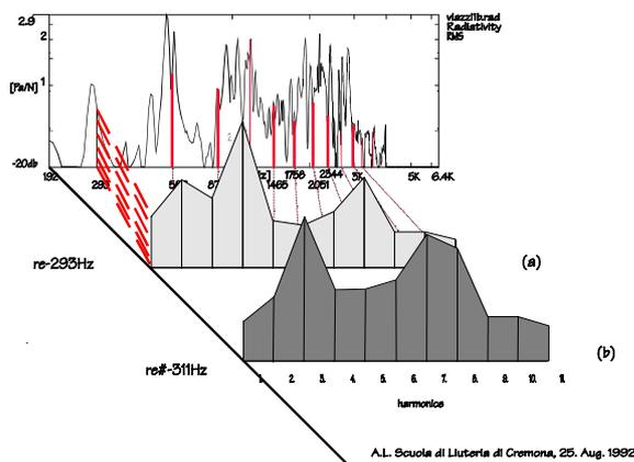
Fig. 3: Grouping together the harmonics of every fundamental frequency results in a easier reading of the acoustic spectrum of the violin.
