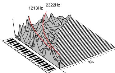
Fig. 4: The 3D plot of the radiativity spectrum of fig. 3. The x-axis represents the frequencies of the playable notes of the instrument. The y-axis represents the number of the harmonics relative to the note on the x-axis. The z-axis represents the amplitude. The same scale is used as in fig. 3.
